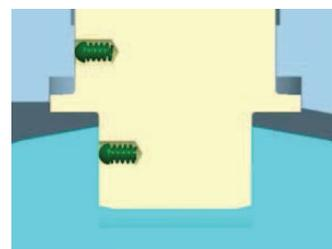
In general, this is achieved through 35% carbon-filled PTFE stem seals and Graphite gland packings to provide electrical continuity between the body and the stem / ball, discharging any build-up of static charge. In addition, spring-loaded plungers are provided between the stem and the ball from DN80 to DN150 (459 Series). Depending on the choice of seals, the designs also provide for additional spring-loaded plungers between the stem and the body for full mechanical antistatic capability.
