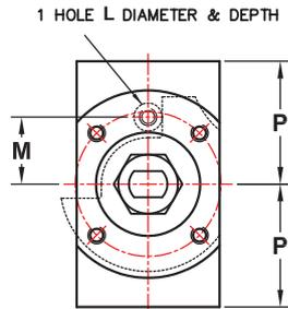
4 BOLT FIXING (DN32 - DN50)
