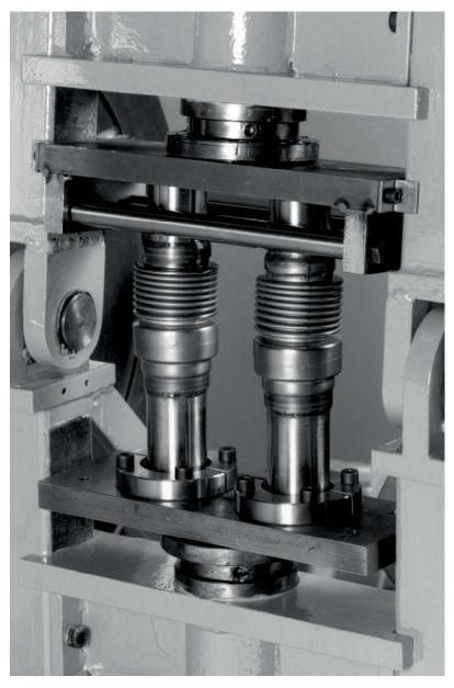
We manufacture expansion bellows mostly of austenitic stainless steel SA240 grade for thin wall metal sheets and coils. This material having high modulus of elasticity and corrosion resistivity is preferred for bellow manufacturing. In line with austenitic stainless steel other alloys of nickel base are also used in bellow application.
