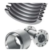
Our thin wall single layer or single ply work more effectively for low pressure and vacuum application. Due to low spring rate this bellows are more adaptive to flexibility and are convenient for compensating combined movements and vibration isolation.
