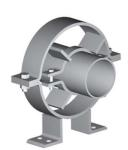
Pipe guides are basically installed for alignment and balancing of pipes in motion. During thermal expansion pipes undergo different movement like axial, transverse or angular movements. Pipe guides are mainly installed in-line with expansion joints. As they provide specific direction to pipe, this makes expansion joints to work effectively and also increase life of expansion joints. We design and supply pipe guides as per piping engineer recommendation.
